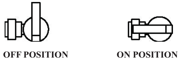
TOP VIEW OF TANK BALL VALVE (PPSV501222W)
